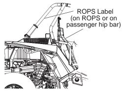
nets or doors, the ROPS helps prevent occupants from being ejected from the vehicle. Always follow all safe operating practices outlined in this manual to avoid vehicle rollover.
