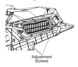
6. Tighten or loosen the three (3) headlight screws on the rear of the headlight to adjust the beam upward or downward or to the left or right.
