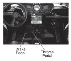
**Tip:** If the throttle pedal and brake pedal are applied simultaneously, engine power may be limited.
