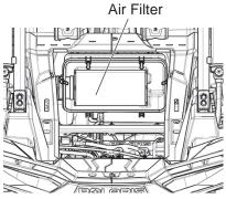
7. Reinstall the air filter (if clean) or install a new air filter (if soiled). Do not attempt to clean the air filter.
