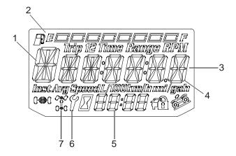
1. **Gear Indicator** - This indicator displays gear shifter position.
