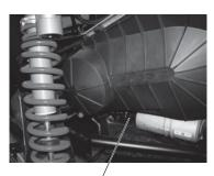
Rear Prop Shaft Grease Fitting
